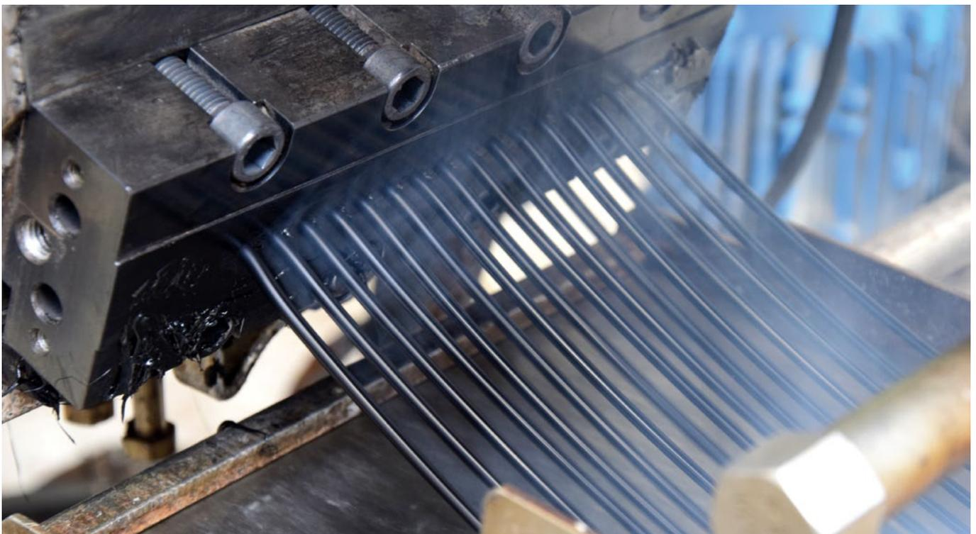
The powdered raw material is processed with the addition of additives in a new extrusion process into a quality recompound from which new products can be manufactured.
